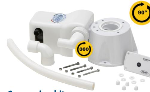
Converts compact and comfort bowl of most toilets with 4 bolt fixing bowls and bolt centres on a 95 mm (3 3/4") diameter circle such as Matromarine, Jabsco, TMC, Raritan, RM69, Johnson Pump, Theford, Lalizas. Included kit contains all necessary parts, such as stainless steel bolts and washers, hose and gaskets and control panel. Space saving thanks to the possibility of rotating 90 degrees the pump and provided accessibility for servicing
