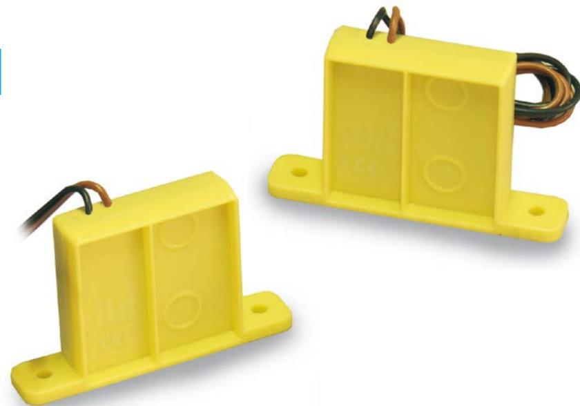
This EMD switch senses water level and automatically controls a 12-to-24 volt bilge pump. It turns on when it senses 51 mm. water level and turns off when water is below 19 mm. Ignition protected. CE certified.
