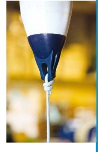
Breakage tests of injection ropeholders always performs up to 1 ton of weight.
